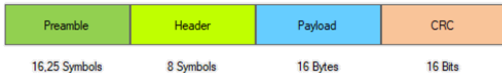
Figure 13. LoRa Packet Format of the Purpose of our interference immunity study
