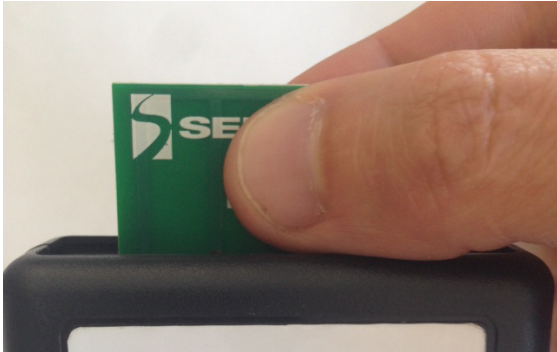
Figure 2-7: Press the Antenna to Enter Bootloader Mode
